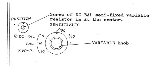
Adjustment of horizontal axis DC balance Conduct this adjustment 15 to 20 minutes after the 552H is energized.
