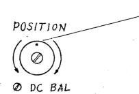
The knob is in the middle of its turning range when the white dot or line, on the knob is at the top.
